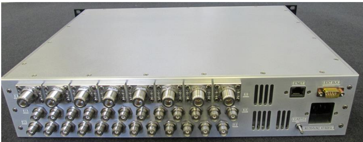
REAR PANEL VIEW - USC410 MATRIX SWITCH ( TNC INPUT and OUTPUT CONNECTORS )
