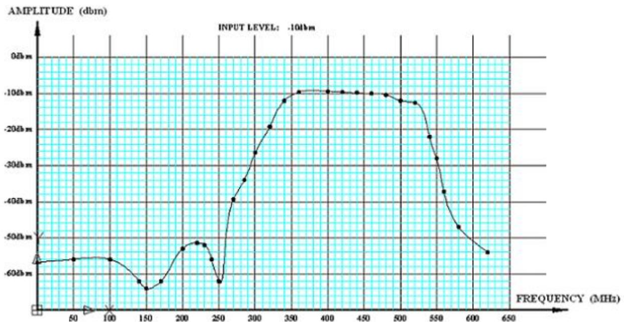
**2. Sensitivity Control:** The Pre Amplifier Module includes a 'Sensitivity' control. This comprises an in line 15db Attenuator that can be switched into circuit to provide a de-sensitised input, or out of circuit to provide normal sensitivity. This extends the linear operation of the system to +15 dbm at the input.
