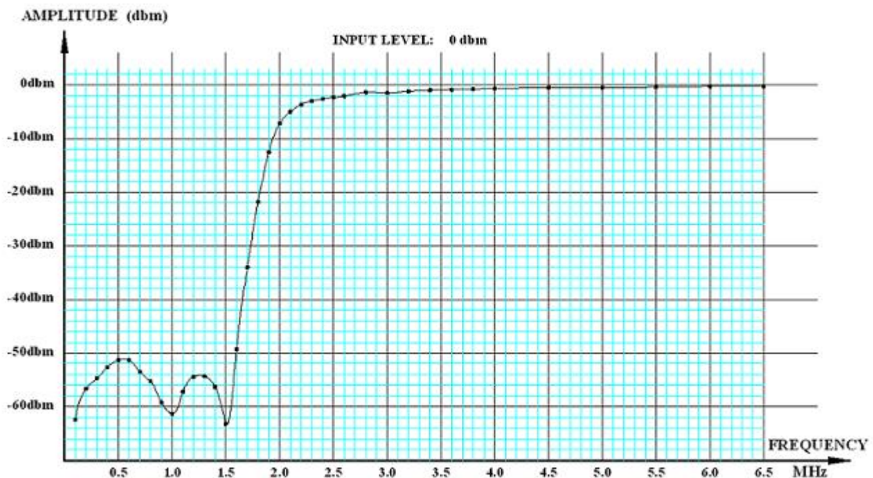
A TYPICAL HF BAND HIGH PASS FILTER RESPONSE (CORNER FREQUENCY 2.2 MHz)
