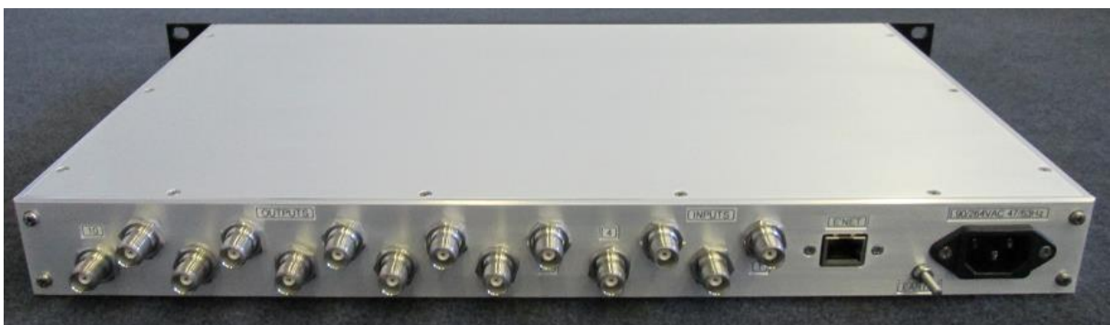
REAR PANEL VIEW - USC410 MATRIX SWITCH ( TNC INPUT and OUTPUT CONNECTORS )
