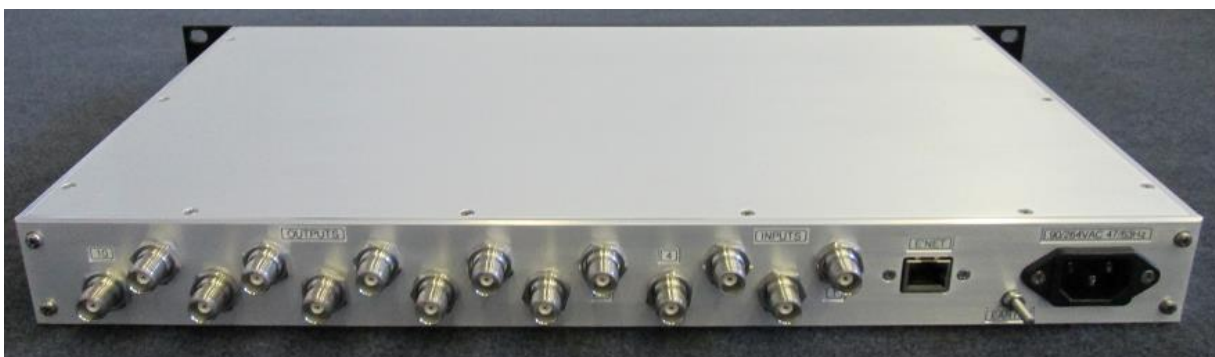
REAR PANEL VIEW - USC410 MATRIX SWITCH ( TNC INPUT and OUTPUT CONNECTORS )
